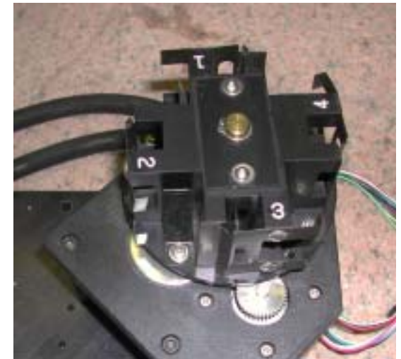
4 Position Turret SPEX Fluoromax-2, Jobin-Yvon
